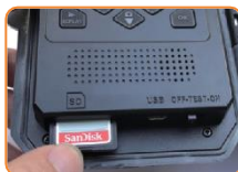
2. Instalar tarjetas SD
